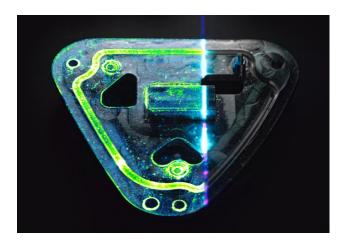
Organic substances fluoresce in laser light. The F-scanner scans the entire component surface in a matter of seconds, seamlessly detecting even the slightest contamination. © Fraunhofer IPM
