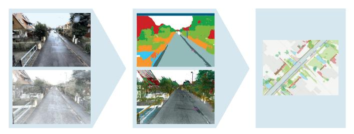
2D camera data (upper left) and 3D laser scanner data (lower left) depict the infrastructure quickly and efficiently. 3D-AI analyzes the data automatically using smart algorithms (mid). Each color in the point cloud represents a singular class of objects. This data is then transferred to a digital planning map (right) for automated route planning. In addition to the categorized surfaces, this plan contains information on the position of the objects.
