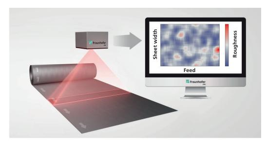
The R-Imager inline inspection system can be easily integrated into existing production processes thanks to its large working distance.
