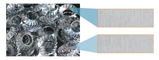
Each punched part is characterized by individual microstructures on its surface. Track & Trace Fingerprint Inline reduces these structures to a simple bit sequence.
