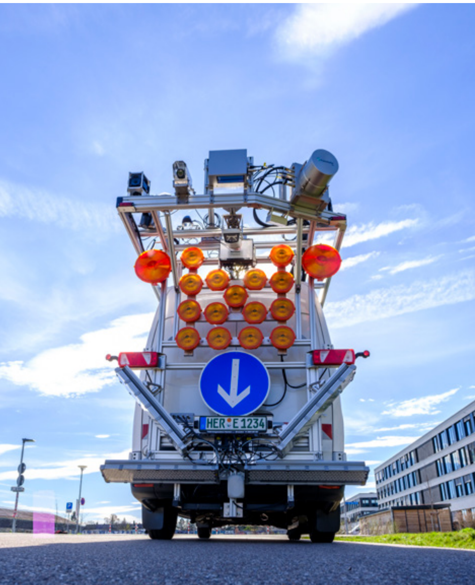
Highly sophisticated measurement technology: A universal vehicle records the state of the road surface while capturing the street environment at the same time.
