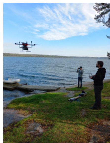
Finnish researchers test the ultra-lightweight bathymetry laser scanner.
