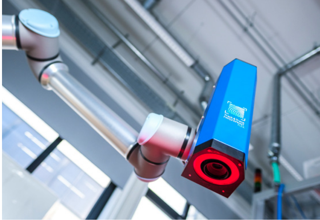
Track & Trace Fingerprint Flex on a robotic arm: The system identifies components and can be used anywhere in the production environment.
