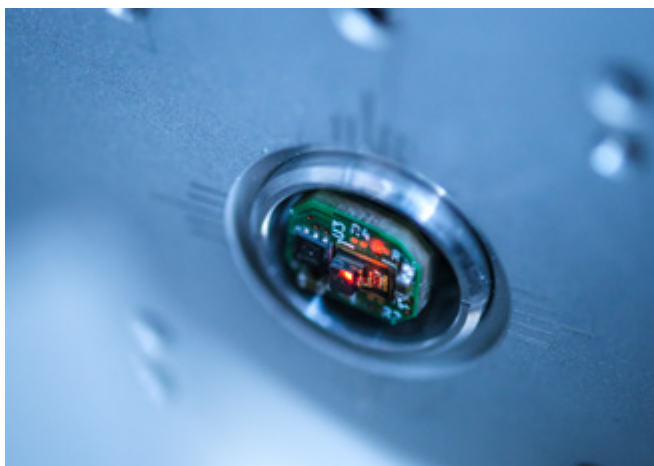
A photoacoustic CO 2 detector is characterized in a spectrometer setup.
