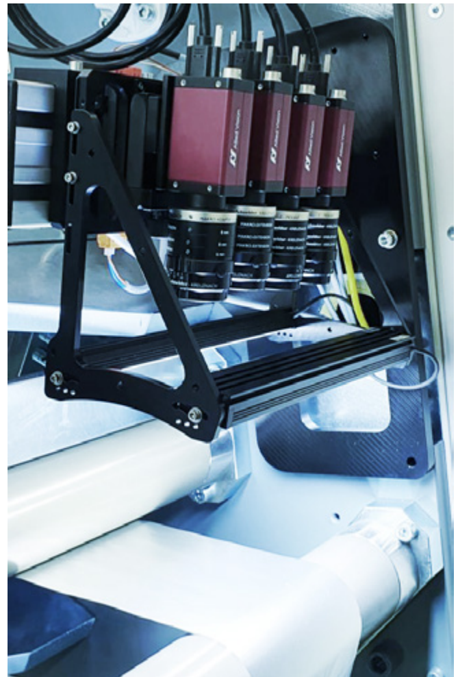
Reliable tracing of sections: In the production of sheeting, process data can be linked to a specific section of a coil with Track & Trace Fingerprint technology.
