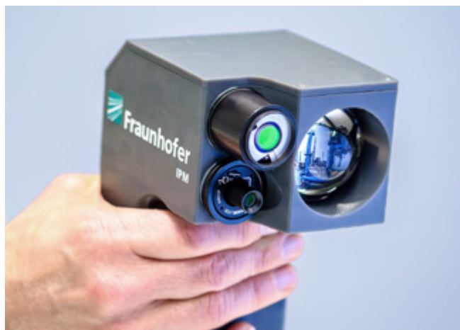
A handheld laser-based spectrometer for remote gas detection measures ammonia leaks using a contactless technique from distances of up to 50 m.
