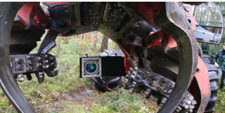
The Track & Trace Fingerprint system captures the cut surfaces of tree trunks on the forest harvester.
